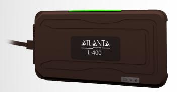
Atlanta L-400 is a smart 4G Basic vehicle tracker with internal high-gain LTE & GSM antennas and integrated credible battery backup. It has 4 digital input which can be used for ignition, door, or alarm button status monitoring & 1 digital output which help achieving vehicle in can remote immobilization.
